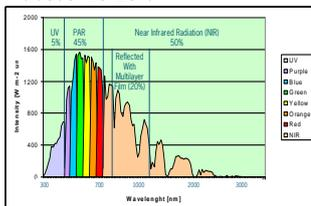
Fig. 2 The AM 1.5 Solar radiation. Radiation between 800 - 1200 nm is reflected by the multilayer film on the lamellae.
