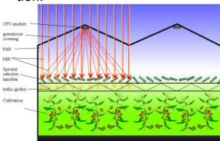
Fig. 1 Working principle of the lamellae greenhouse: the lamellae performed as a Fresnel mirror and reflect the direct solar Near Infrared Radiation (NIR) onto the PV-module. (visible light → and NIR radiation →)
