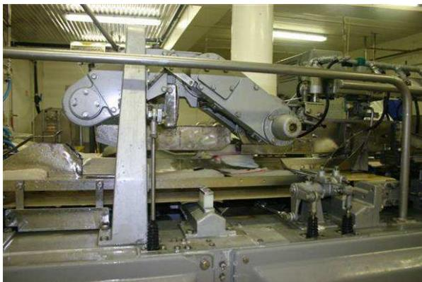
**Figure 3** Machine filleting cod
