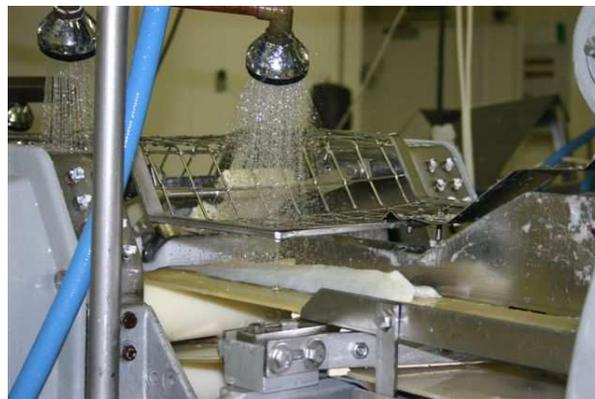
**Figure 4** Machine filleting cod
