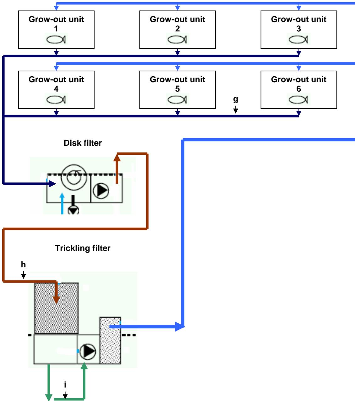
Figure S2: Flow scheme of system C/D. The different colors dark blue, brown, green and light blue correspond to the different sampling points in the following order; Outlet grow-out unit (g), Outlet disk filter (h) and Outlet trickling filter (i).
