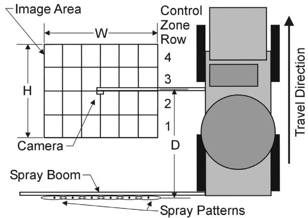
**Figure 2.** Physical configuration of the image area and spray nozzles. The image is divided into six columns and four rows of control zones, resulting in a 2.44 m high  $\times$  3.05 m width usable image area. The camera was mounted 3.09 m ahead of the spray boom.
