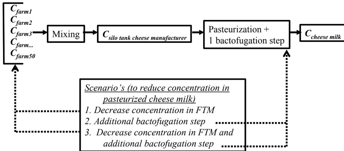
**Figure 8.3** Standardized process for the production of pasteurized cheese milk with scenario's to reduce the butyric acid bacteria (BAB) spore concentration in pasteurized cheese milk.
