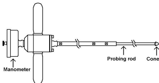
**Figure 3.2** Schematic representation of hand penetrometer (Eijkelkamp Agrisearch Equipment, Giesbeek, The Netherlands)
