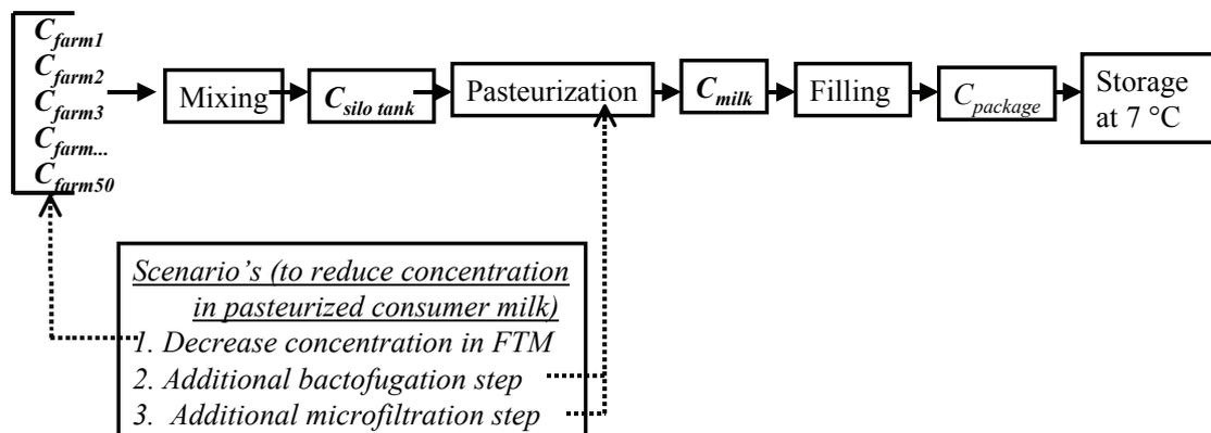
**Figure 8.4** Standardized process for the production of pasteurized consumer milk with options to reduce the *Bacillus cereus* spore concentrations.
