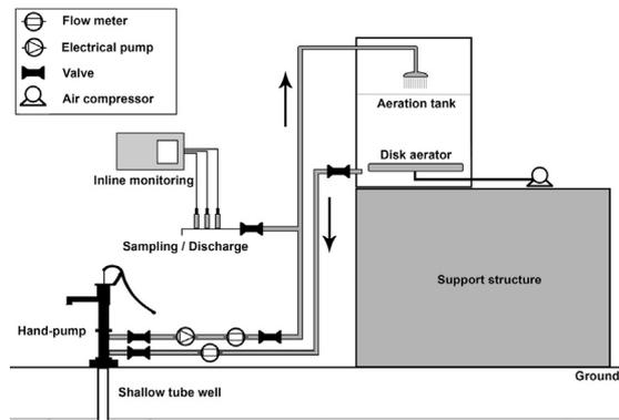
Fig. 2. Prototype of sub-surface arsenic removal technology [8,29].
