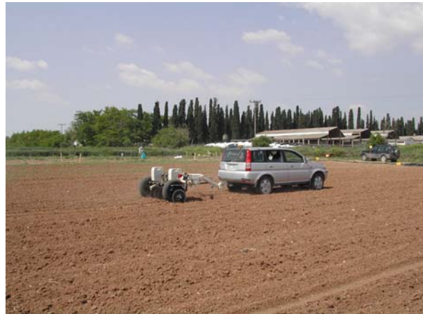
Figure 5. The VERIS® 3100 system including a GPS and joined in 4X4 car for measurements of soil’s apparent electrical conductivity at 30 and 90 cm depths in the AFS study field
