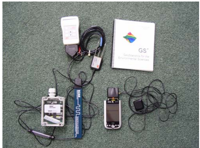
Figure 6. A set of sensors, data loggers, GPS and software used for soil continuous or point data acquisition and analysis
