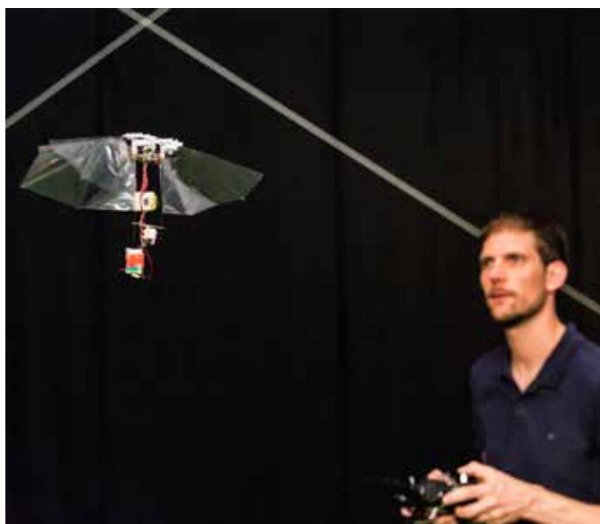
DelFly Nimble in stationary (hovering) flight. Foto TU Delft.
