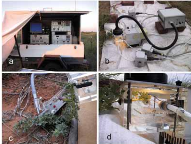
Figure 6. a: Arrangement of modules and controlling unit of the gas exchange measuring system under Kalahari conditions; b: view onto the cuvette with dew-point mirrors and fibre illuminator; c: arrangement of leaf clip and measuring chamber at simultaneous measurement of gas exchange and chlorophyll fluorescence; d: detailed view into the measuring chamber
