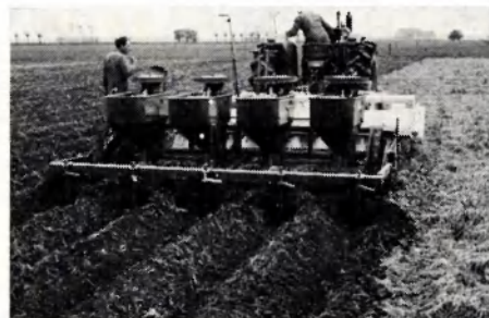
Fig. 4 A rotavator with times together with a potato planting machine (van Rump NV).
