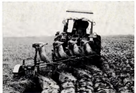
Fig. 6 Modern mould-boards and their work (Fa. Iz. Cappon).
