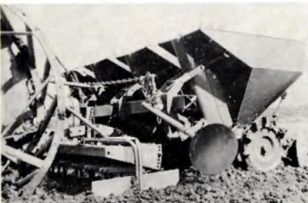
Fig. 3 A combination of a horizontal rotating powered harrow and a planting machine (van der Lely NV).
