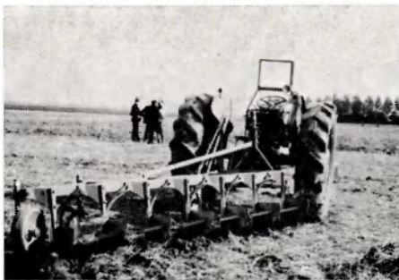
Fig. 5 The stubble plough (van Rumpt NV).
