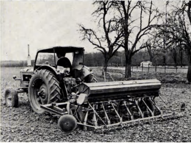
Fig. 2 A four-bar-powered harrow combined with a seed drill (Vicon NV).
