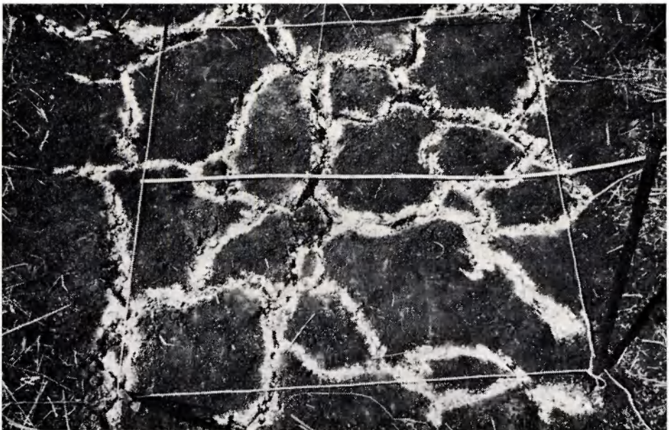
Fig. 1 Cracking pattern of a grumusol indicated by talk powder on 1 m 2 , prior to tillage.
