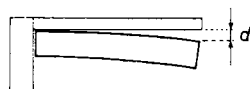
FIG. 5 THE MOST PRACTICAL METHOD OF MEASURING BENDS ALONG THE CENTRE LINE AND NOT STRAIGHT CUTS OF THE TILES. THE DISTANCE d IS TO BE INTERPRETED AS A DISPLACEMENT.
