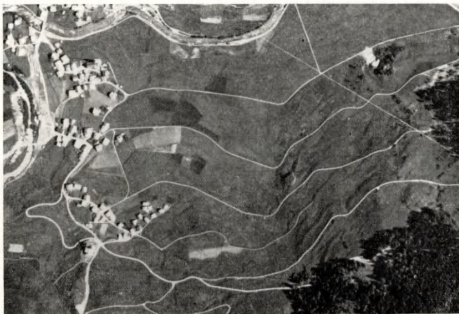
FIG. 2b IDEM, NEW SITUATION. ROADS ALONG THE CONTOUR LINES. Aerial photographs of the Eidg. Landestopographie. All rights reserved. Consent of 13.2.1956.
