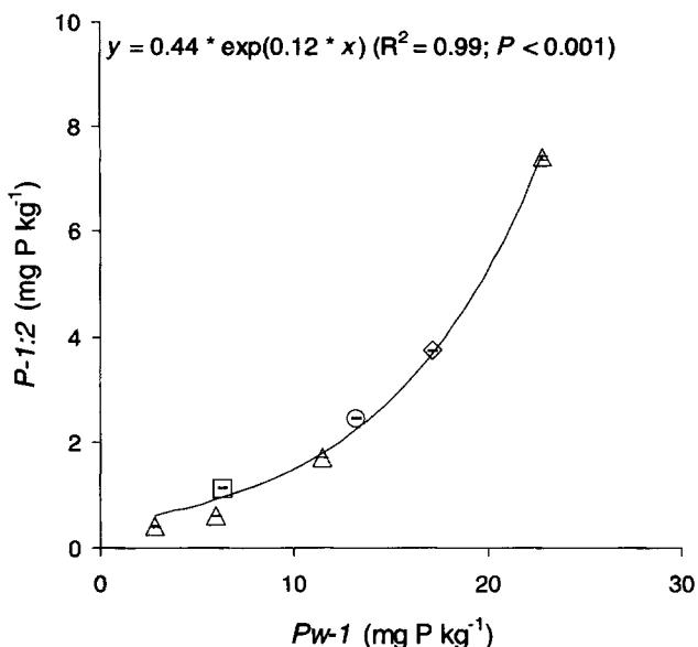
Figure 3.  $P_{w-1:2}$  (water-extractable P at a soil:solution ratio of 1:2 w:v) versus  $P_{w-1}$  (water-extractable P at a soil:solution ratio of 1:60 v:v) for the soils studied. Means with sample standard deviation of  $P_{w-1:2}$  ( $\diamond$ : Emmer C.;  $\square$ : Giethoorn;  $\triangle$ : Haren;  $\circ$ : Wijster).
