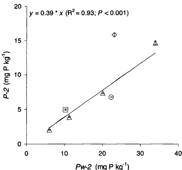
Figure 2.  $P-2$  (0.01 M  $\text{CaCl}_2$ -extractable P at a soil:solution ratio of 1:60 v:v, end-over-end shaking) versus  $Pw-2$  (water-extractable P at a soil:solution ratio of 1:60 v:v, end-over-end shaking) for the soils studied (line fitted for the results of all soils excluding Emmer C.). Means with sample standard deviation of  $P-2$  ( $\diamond$ : Emmer C.;  $\square$ : Giet-hoorn;  $\triangle$ : Haren;  $\circ$ : Wijster).
